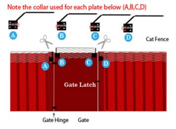
Set Arms "B" and "C" above Arms "A" and "D" so that when the gate opens outward the Arms on the gate ("B" and "C") will pass ABOVE the fence material and Arms ("A" and "D") on either side of the gate. Test opening the gate before you add the Fence material to be sure that the Arms do not hit each other, preventing the gate from opening. Cut the fence between Arms "A" and "B" as well as "C" and "D".
